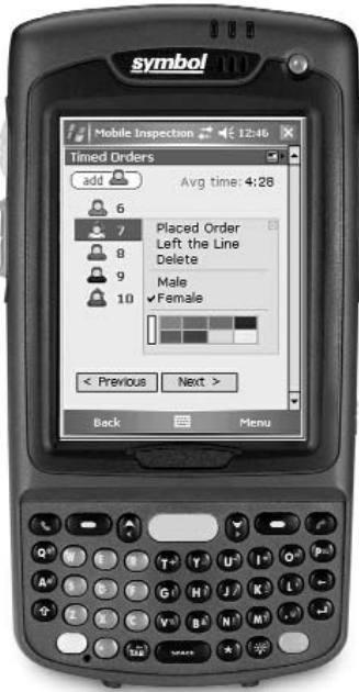
Mobile inspection application on a PDA showing a customized question type designed for timing service operations.
