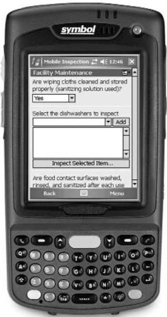
Mobile inspection application on a PDA showing standard question and answer types generated using the forms builder.
